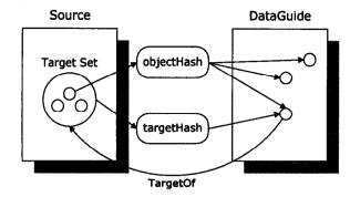
Figure 5. Data structures for DataGuide maintenance
