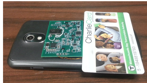
Figure 11: Our EnGarde prototype meets the form factor needs required for semi-permanent attachment to a mobile phone. Here, we show it on the back of a Galaxy Nexus
